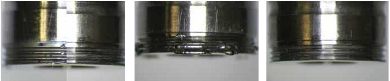
Above are the two side-by-side inserts showing damaged threads (left); one insert during laser welding repair work (middle) and the same insert after repairs and polishing were complete (right).
