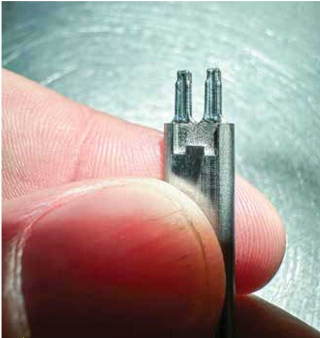
Laser welding offers a host of benefits for tool and die repairs over TIG welding.
