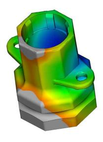
Key technologies like laser scanning and mold flow analysis to help identify potential performance issues.
